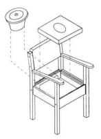
**Step 4.**Place the fibre glass seat (14) in the frame resting upon the support bars.
