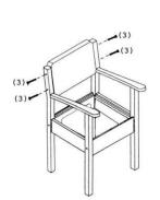
Step 3. Fit the back rest (12) to the sides by using 4 pcs of 6x45mm JCBC screws (3).
